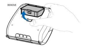
Remove the battery as shown.
