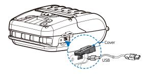
${\bf 1} \quad {\sf Flip \ over \ the \ connector \ cover \ and \ connect \ {\sf USB \ cable \ to \ the \ printer \ connector.}}$
