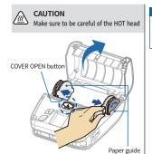
Place the paper roll as shown. Make sure the paper is placed in the right direction.
