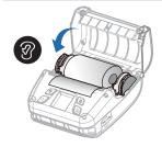
Pull a short length of paper out of the printer and close the cover.
